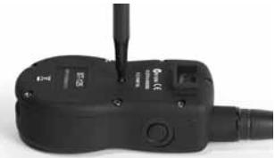
For example, if mode 2 is desired, adjust the Intensity Dial to Level 2. Once the Mode Button has been depressed, the Transmitter Indicator Light will be solid and, once the mode button is released, the Transmitter Indicator Light will flash 2 times.
